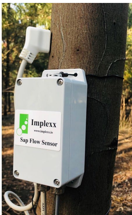
Implexx Sap Flow Sensor Gen1 model includes the grey box and the probe spacing is 0.6 cm.
