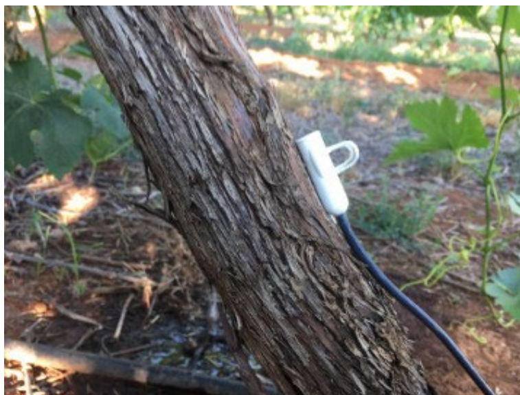
Figure 2. Probe misalignment can occur even when extreme care is taken with drilling and the installation process. Grapevines, such as seen here, can be difficult as well as installing a sensor where the trunk is at an unusual angle.
