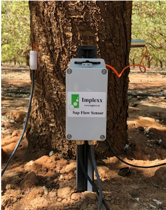
Figure 2. The Implexx Sap Flow Sensor provides in-situ, non-destructive and continuous estimates of stem water content as well as sap flow and stem temperature.
