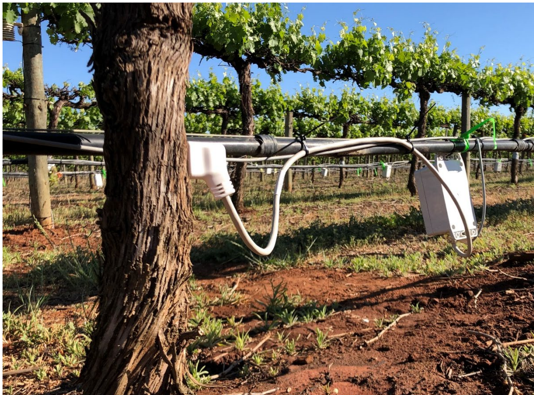
Figure 1. The Implexx Sap Flow Sensor, installed here on a grapevine, measures sap flow, water use or transpiration.
