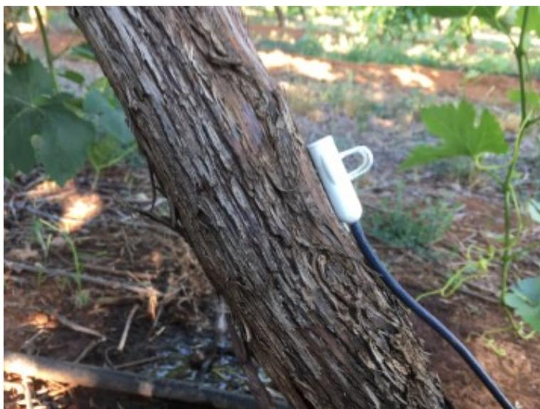
*Figure 2. Probe misalignment can occur even when extreme care is taken with drilling and the installation process. Grapevines, such as seen here, can be difficult as well as installing a sensor where the trunk is at an unusual angle.*
